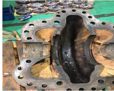
Gambar 4.11 Proses cleaning casing (Sumber : PT.Chandra Asri Pacific)
