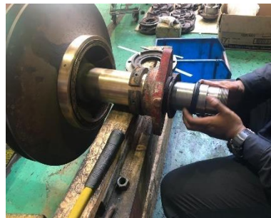
Gambar 4.10 Proses pemasangan seal ring (Sumber : PT.Chandra Asri Pacific)
