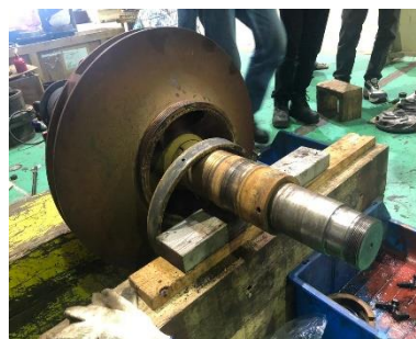
Gambar 4.3 Disassembly Wearing ring lama (Sumber : PT.Chandra Asri Pacific)
