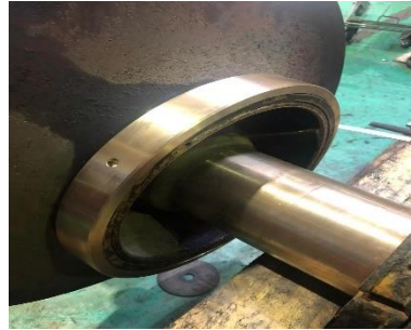
Gambar 4.4 Assembly Wearing ring baru (Sumber : PT.Chandra Asri Pacific)
