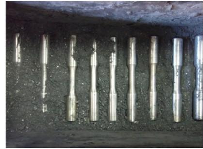
Fig. 2. ASTM E-466 standard test samples
