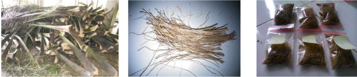
Figure 2. Fiber separation of oil palm empty fruit bunches
