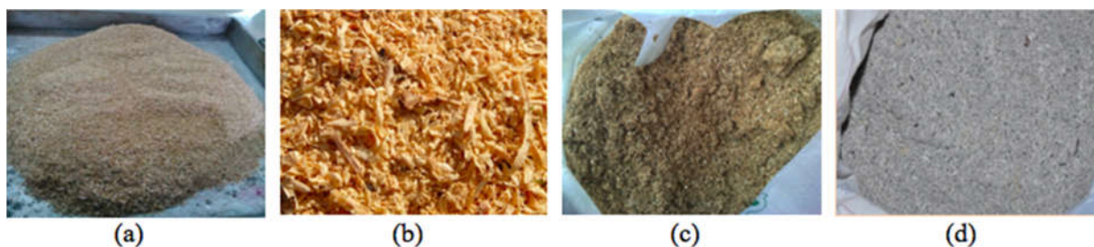
Figure 1. Filler from wood (a) sengon, (b) mahogany, (c) bayur, and (d) rice husk ash
