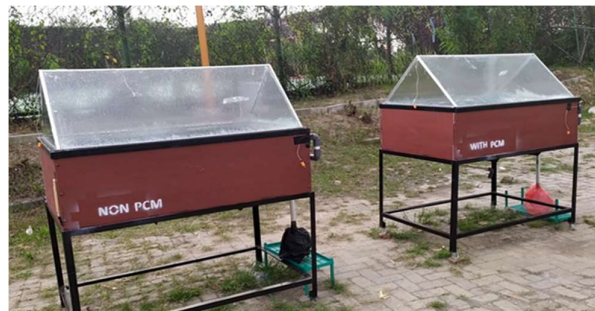
Figure 2. Two similar of solar distillation systems without PCMs and with PCMs
