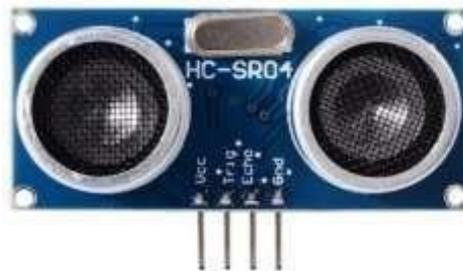
Gambar 4. Sensor Ultrasonik
