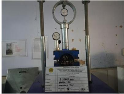
Gambar 5.16 Contoh pengujian *marshall* kadar aspal 4,5% abu ampas tebu 4%
