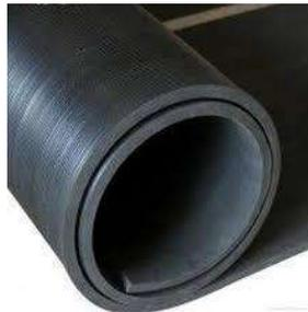
**Gambar 2. 6** Nitrile-Butadiene Rubber (NBR)
