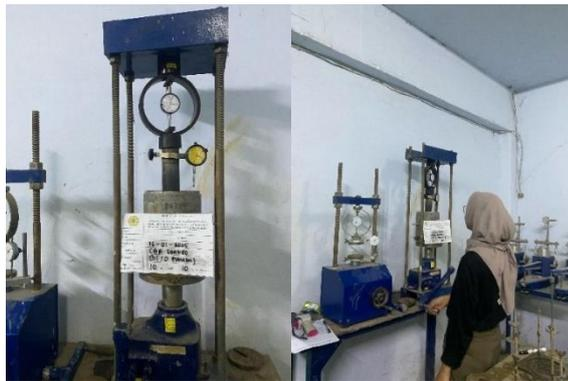
**Gambar 5.22** Pengujian CBR Laboratorium
