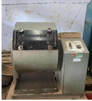
Gambar 4.7 Alat Uji Keausan Agregat (*Los Angeles Abrasion*)
