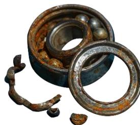
**Gambar 2.8** *Bearing Defect*
