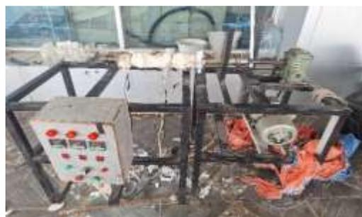
**Gambar 3.2** Mesin *Injection Molding*
