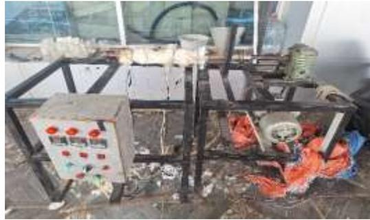
**Gambar 3.17** Mesin *Injection Molding*
