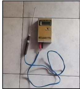
**Gambar 3.8** *Thermocouple*
