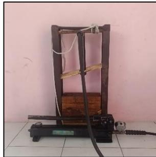
**Gambar 3.7** Mesin *cold press*
