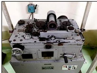
**Gambar 3.11** *Ogoshi high speed universal wear testing machine* [45]
