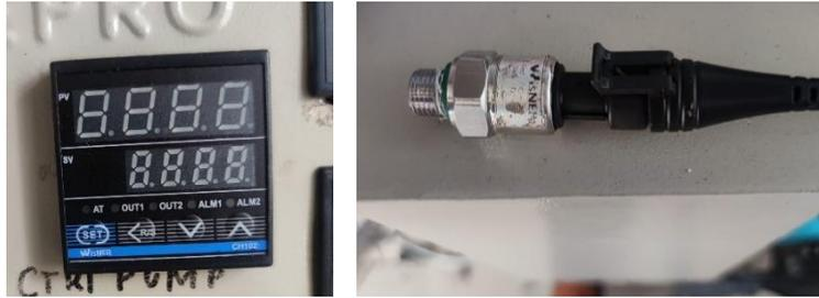
**Gambar 3.8** *Pressure sensor dan Vishner ch102*
