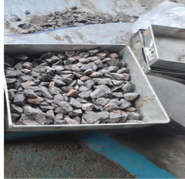
Gambar 5.4 Pengujian Kadar Lumpur Agregat Kasar
