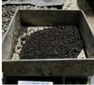
Gambar 5.7 Pengujian Kadar Lumpur Agregat Halus
