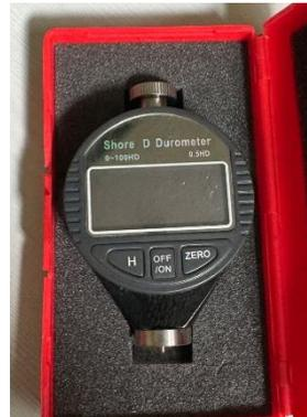
**Gambar 3.10** Durometer *Shore D*
