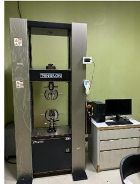
**Gambar 3.5** Tensilon *Universal Testing Machine* RTH-2410
