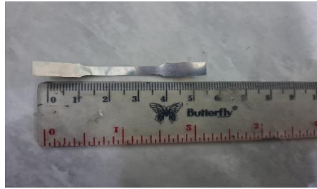
Gambar 3. 2 Spesimen Penelitian Stainless Steel 304
