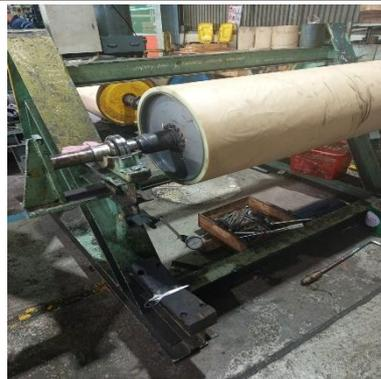
**Gambar 5.3** Proses *Balancing*
