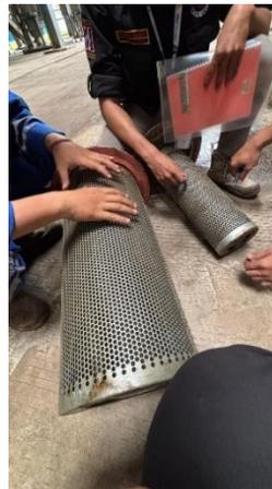
**Gambar 4.10** Proses Pergantian Separator
