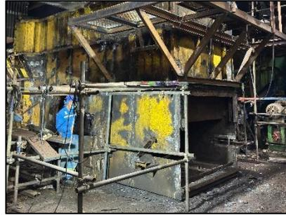
**Gambar 3.9** *Submerged Drag Chain Conveyor*
