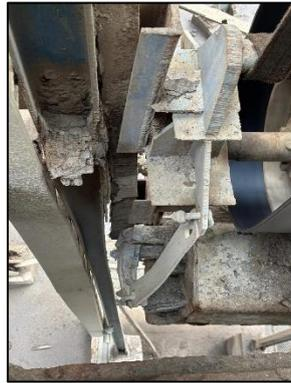
**Gambar 4.6** *Rail Take-Up Pulley* mengalami *Bending*
