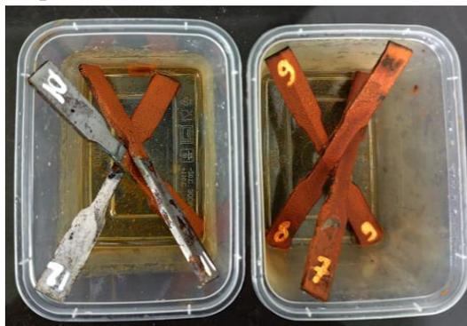
**Gambar 4.11** Material ASTM A36 terkorosi (10 hari)
