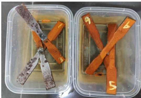
**Gambar 4.12** Material ASTM A36 terkorosi (15 hari)
