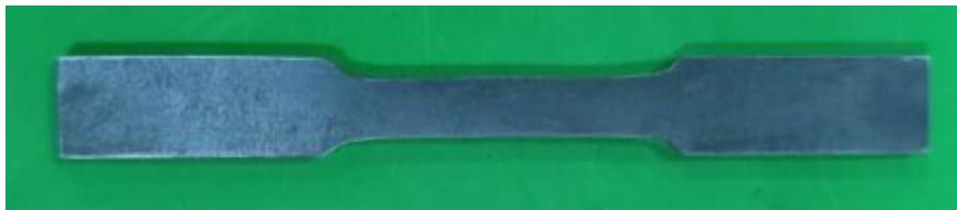
**Gambar 4.2** Spesimen ASTM A36
