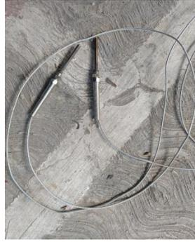
**Gambar 3.12** *Thermocouple*
