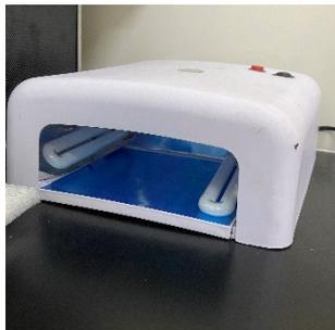
**Gambar C.45** *UV Curing Lamp*
