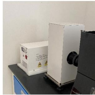
**Gambar C.34** *Solar Simulator*
