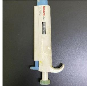
**Gambar C.28** Mikropipet 10-100  $\mu$ l
