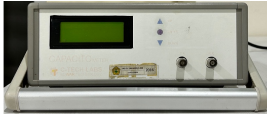
Gambar 2.4 Kapasitometer CAP 3201 2CH C-Tech Labs Edwar
