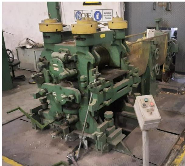
**Gambar C.6 Mesin Canai (*Rolling*)**
