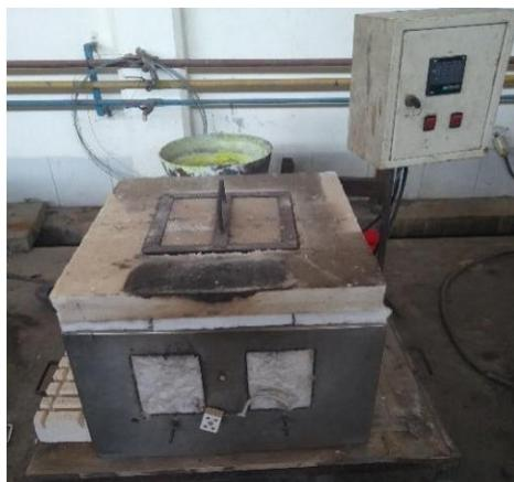
**Gambar C.13** *Muffle Furnace*
