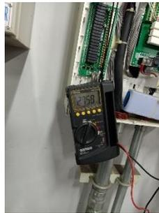
**Gambar 4.13** Pengecekan *Power Supply Unit*
