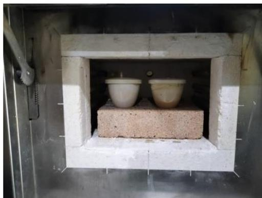
**Gambar 3. 4** Proses *Pack Carburizing*
