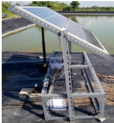
Gambar 2.11 Contoh Solar Tracking Single Axis System [11]
