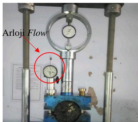
**Gambar 4.11** Alat Uji *Marshall*
