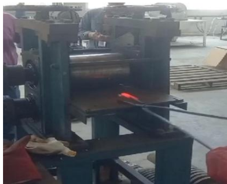
Gambar 3.3 Proses Hot rolling
