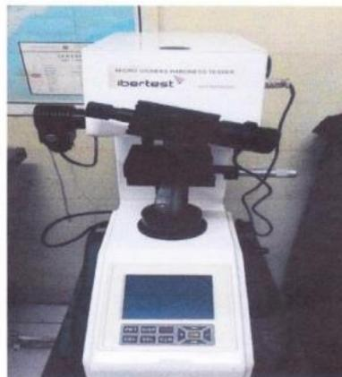
**Gambar 2.6** Uji Kekerasan *Microhardness Vickers*
