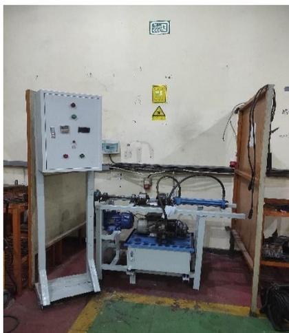
Gambar C.16 Alat *friction welding*
