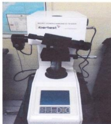
Gambar 2.6 Uji Kekerasan Microhardness Vickers
