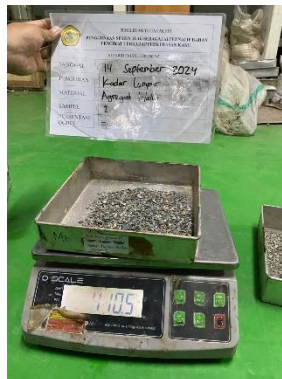
Gambar 5. 10 Pengujian Kadar Lumpur Agregat Halus
