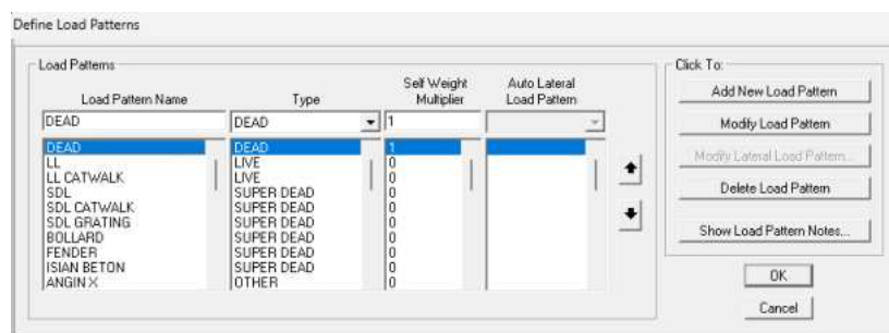
Gambar 12 Define Load Patterns Breasting Dolphin
