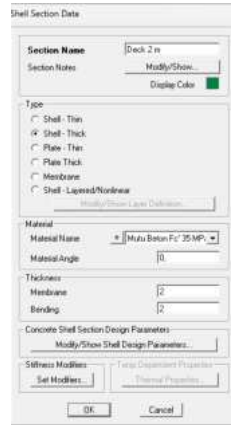
Gambar 52 Slab Property Mooring Dolphin
