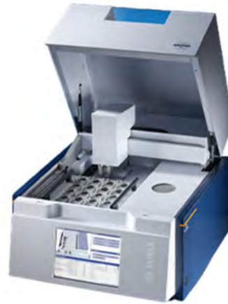
Gambar C.8 Alat Pengujian XRF (Bruker S2 Puma)
