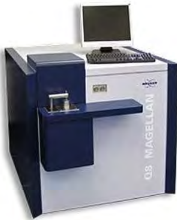
Gambar C.9 Alat Pengujian Arc OES (Bruker Q8 Magellan)
