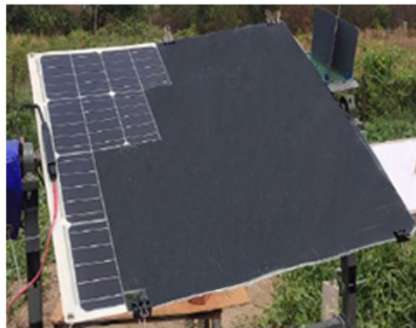
(c) Penutupan 3/4 panel
