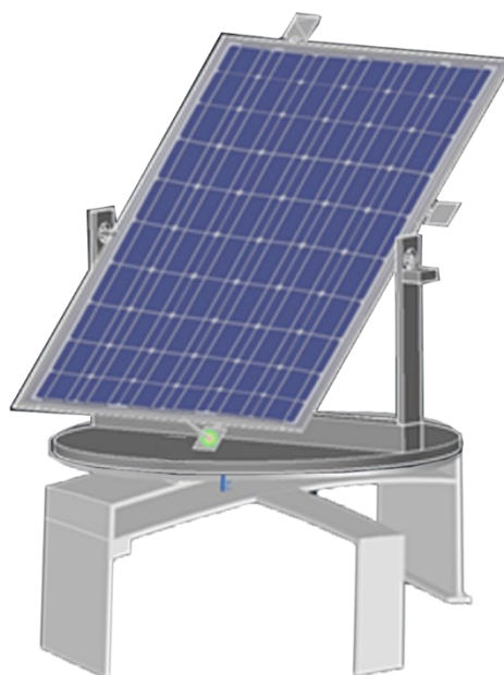
Gambar 3.5 Desain panel surya solar tracking dual axis system
