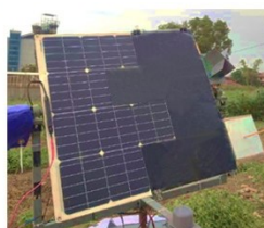
(b) Penutupan 1/2 panel
