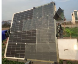
(b) Penutupan 1/2 panel
