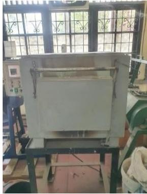
**Gambar C.7** *Muffle Furnace*
