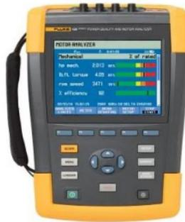
Gambar 3.3 Power quality analyzer fluke 438-II.
