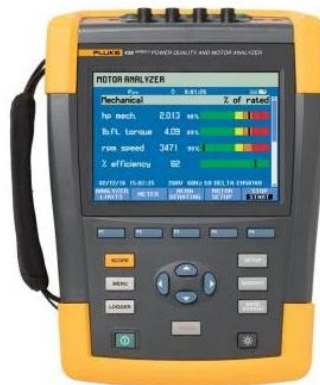
Gambar 3.3 Power quality analyzer fluke 438-II [18].
