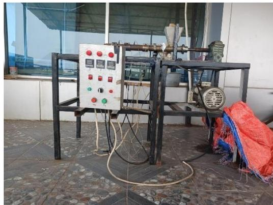
**Gambar 3. 3** Mesin *Injection Moulding*
