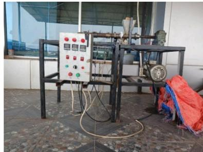
**Gambar 2.1** Injection Moulding
