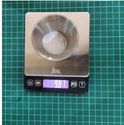
**Gambar 3.19** Proses menimbang alumina
