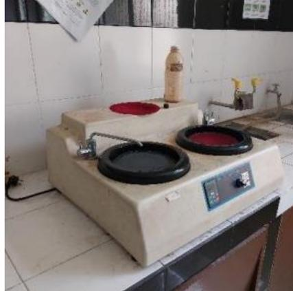
**Gambar 3.15** Mesin *Grinding Polishing*
