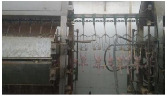
Gambar 2.4 Proses Pencabutan Bulu ( Defeathering )
