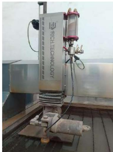
**Gambar 3.14** Mempersiapkan Mesin Water Jet Cutting
