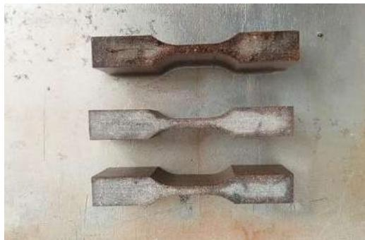
**Gambar 3.18** Spesimen Potong ASTM D638 Section V
