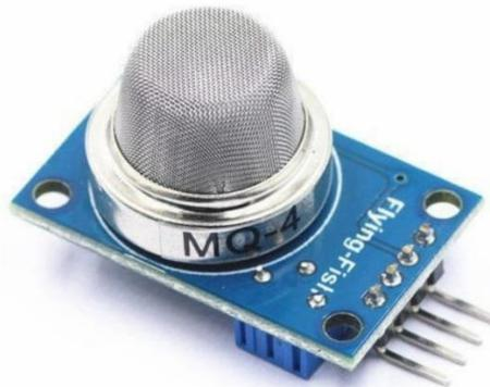
**Gambar 2. 3** Sensor Gas MQ-4 [25]
