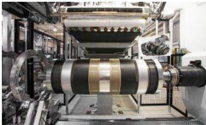
**Gambar 3.5** Drum Karkas di Mesin *VMI Vast*
