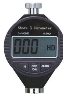
**Gambar 3.3** *Hardness Test Durometer Type D*
