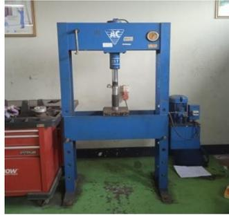
**Gambar 3.8** Mesin Press Hidrolik
