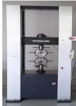
**Gambar 3.2** *Universal Testing Machine RTF Series*
