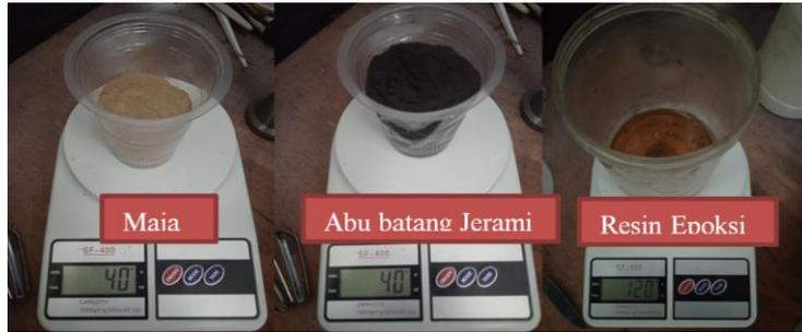
**Gambar 3.34**Proses Penimbangan Bahan Material Kode C
