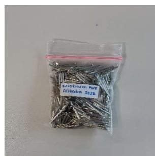
Gambar C.24 Sampel Nb Murni
